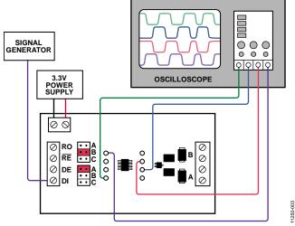
Figure 3. Transmit and Receive Test Setup
